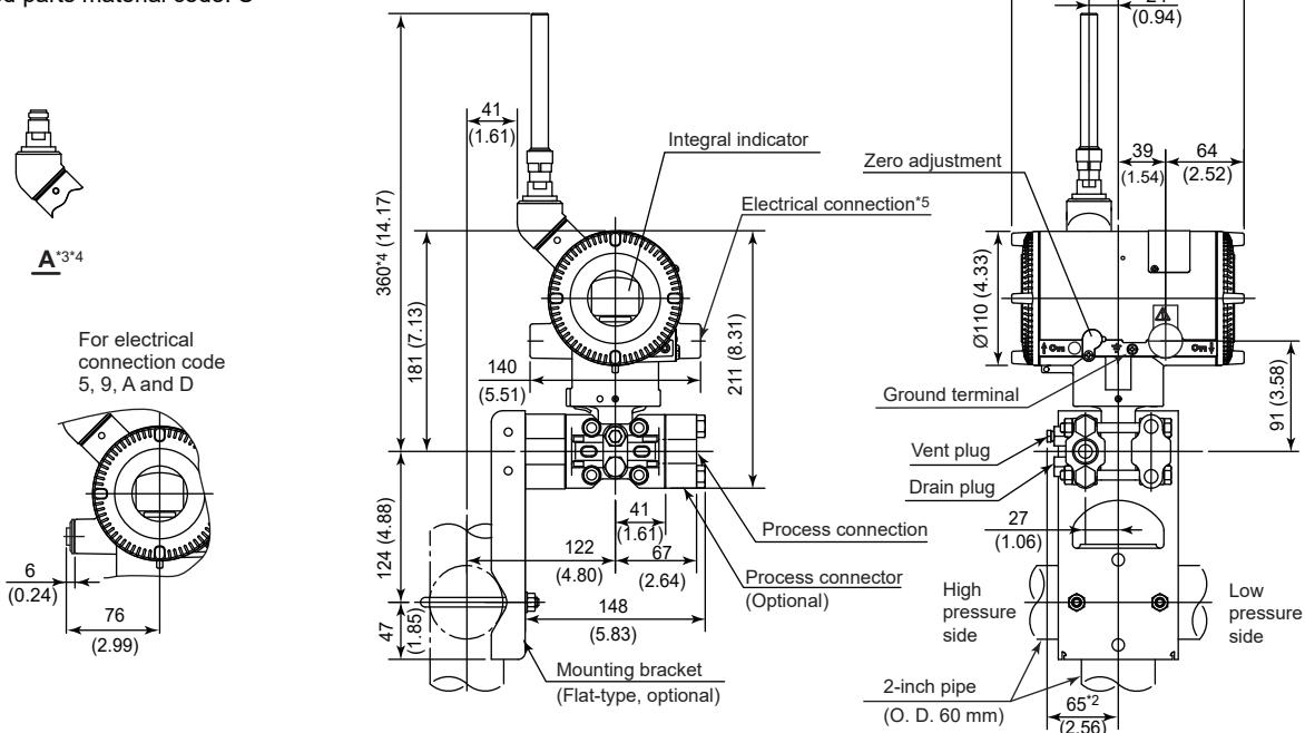
\*1: When installation code -3 and -8 is selected, high and low pressure side on above figure are reversed.
