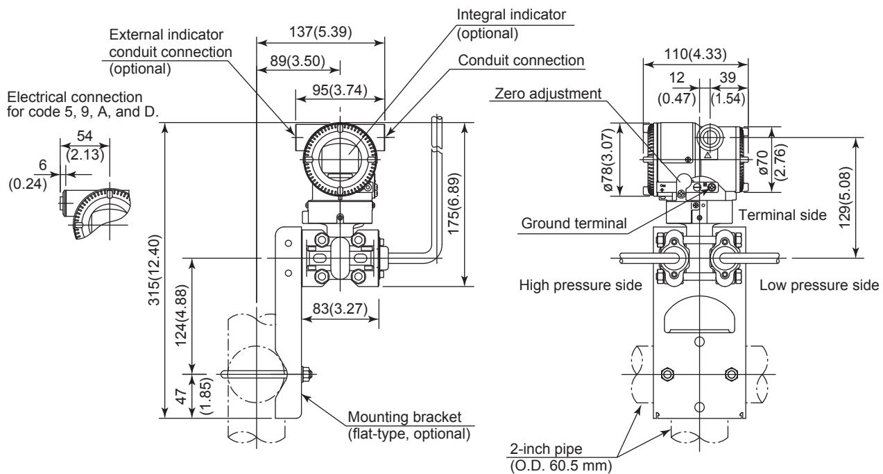
\*1: When electrical connection code 7 or C is selected, a blind plug is protruded up to 8 mm from the conduit connection.
