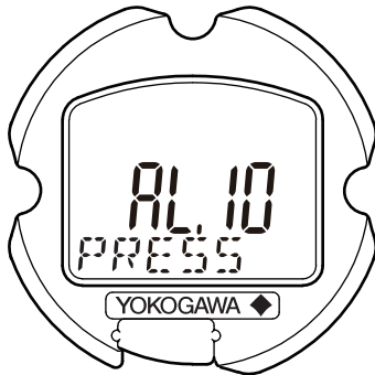
Self-diagnostic error on integral indicator (Faulty transmitter)
