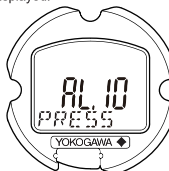
Self-diagnostic error on integral indicator (Faulty transmitter)
