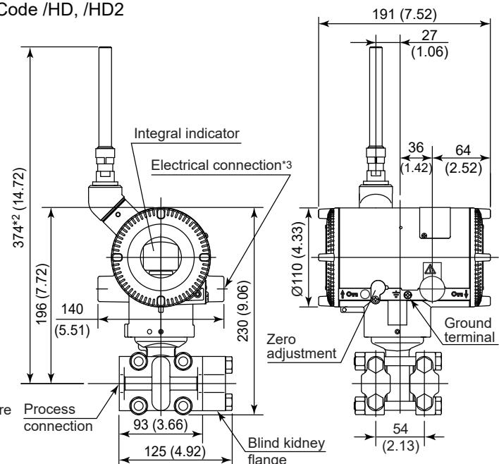
\*1: When amplifier housing code 9 is selected, the value is 240 mm (9.45 inch). In this case, the figure is shown as A.
