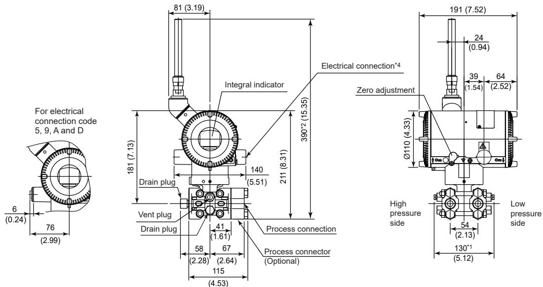
Measurement span code F or option code /HD, /HD2
