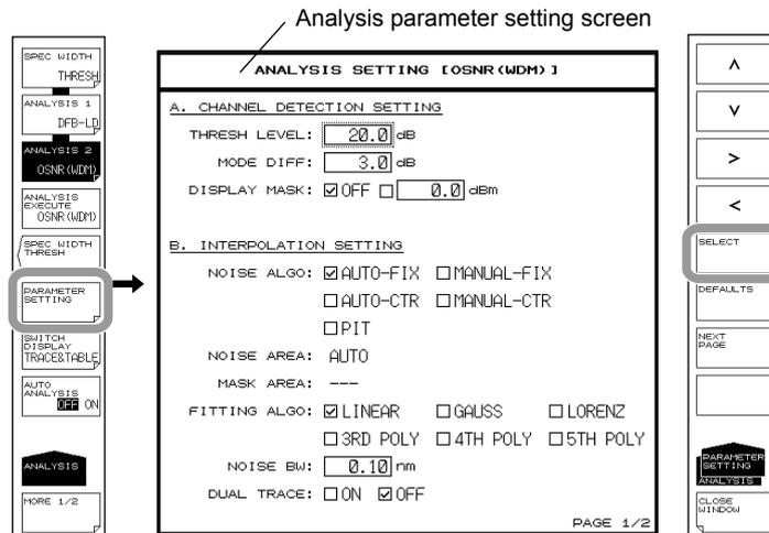
6. Press the **CLOSE WINDOW** soft key. The OSNR (WDM) analysis parameter setting screen closes, and the soft key menu returns to the previous stage.
