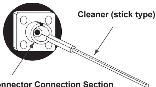
Wiping with a soiled cleaner can damage the optical outputs.
