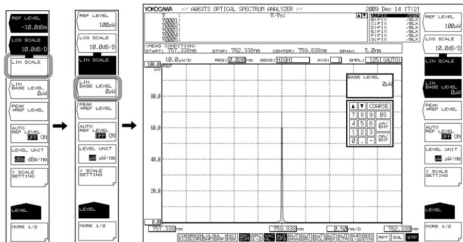
**Setting to Power Spectral Density Display (Setting Units for the Vertical Axis)**
