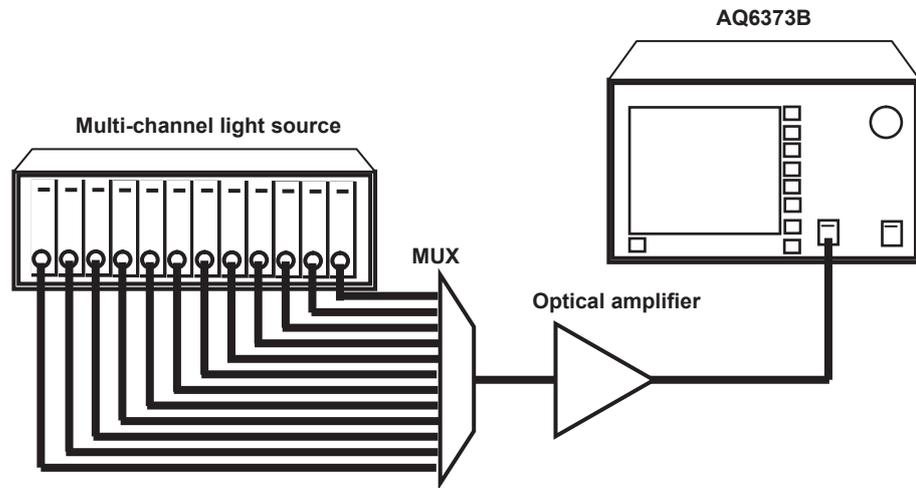
Measure the input optical spectrum and write the waveform to the active trace.
