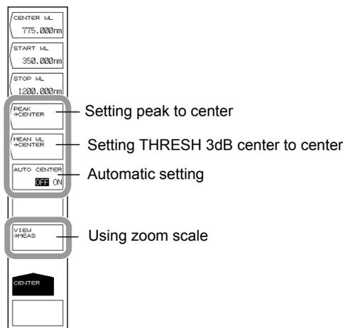
**Also, you can set the wavelength of the moving marker placed on the measured waveform as the center wavelength or center frequency.**
