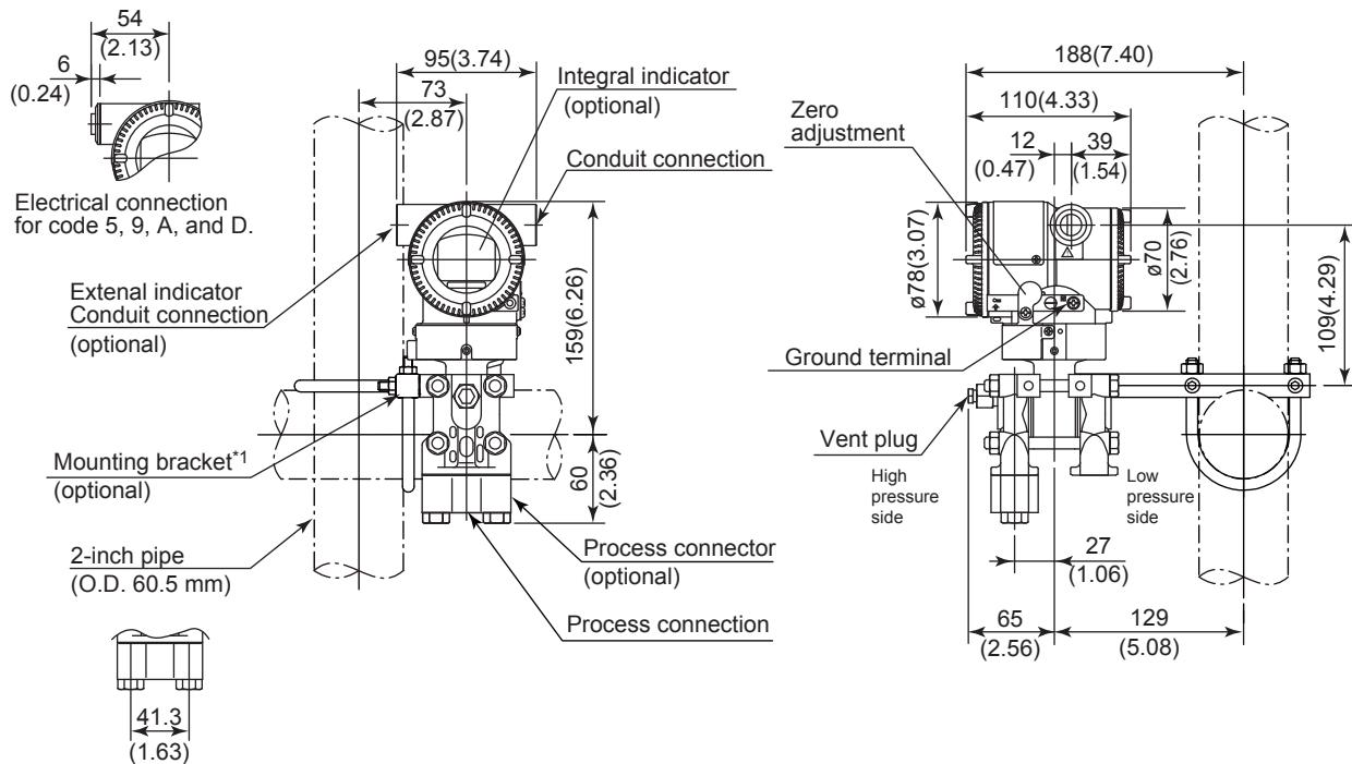
\*1: A transmitter with SST housing is not applicable for mounting to horizontal 2-inch pipe.
