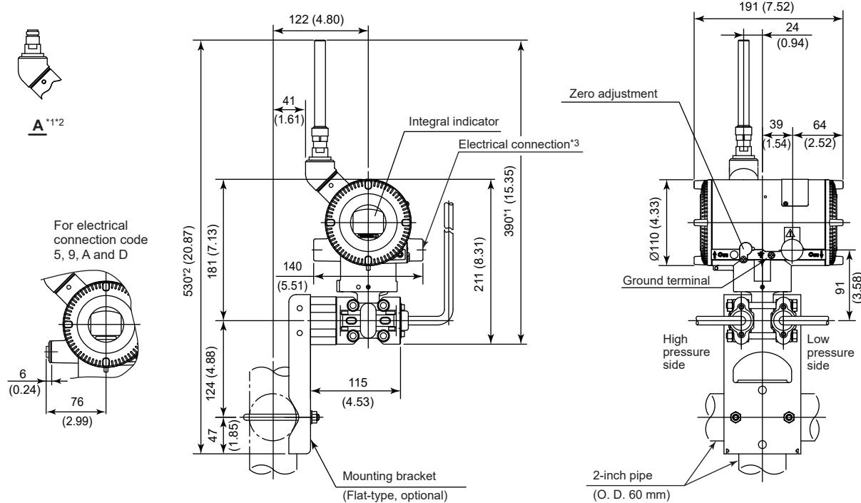
\*1: When amplifier housing code 9 is selected, the value is 270 mm (10.63 inch).
