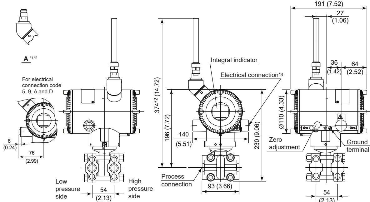
\*1: When amplifier housing code 9 is selected, the value is 240 mm (9.45 inch). In this case, the figure is shown as A.
