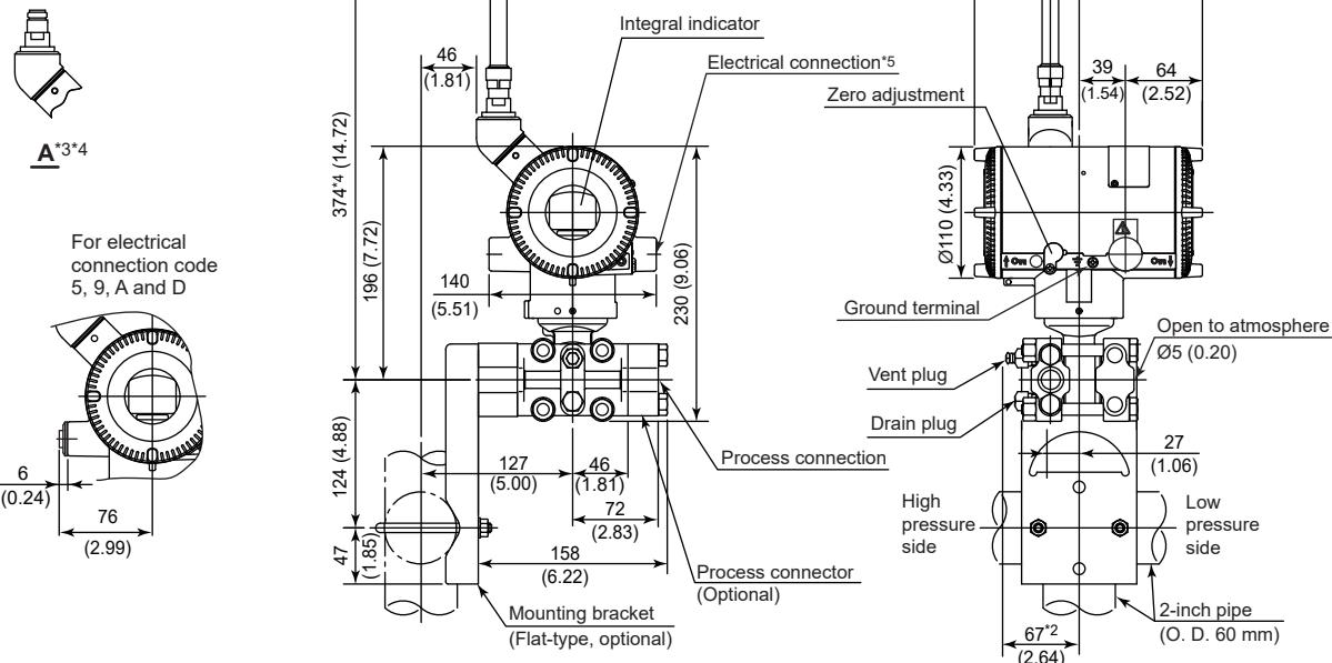
\*1: When installation code -3 and -8 is selected, high and low pressure side on above figure are reversed. (i.e. High pressure side is on the right side.)
